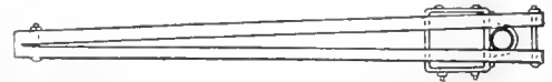
Fig. 9. Top View of Temporary Arm Rigging. This Arm Straddles the Pipe and is Securely Guyed at the Rear
